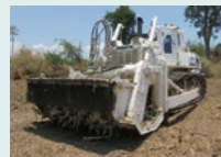
An anti-personnel landmine removal machine
