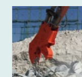
Secondary crusher (G200) equipped with booster
