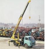
Aichi Sharyo(currently Aichi Corporation) AC-D4Edigger derrick / pole setter(1966) This vehicle consisting of a derrick fitted to a pole setter was a modified version of AC-D4 pole setter.
