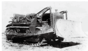
Komatsu D50A bulldozer (1947) This bulldozer, 8t in weight and with a capacity of 55 horsepower, was developed based on a prototype made during the war. Having experienced many breakdowns in initial machines, numerous modifications were subsequently implemented.
