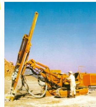
Furukawa Kogyo (currently Furukawa Rock Drill) HCR200 crawler drill (1977) The first domestically manufactured hydraulically operated crawler drill. From around 1983, an era of all-hydraulic drills began on a full scale.
