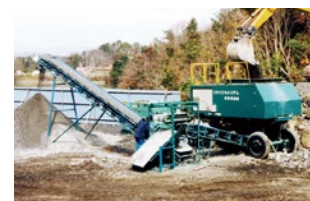
Okada Aiyon PCP-S001 self-propelled crusher (1987) Japan's first self-propelled crusher for use at demolition sites.
