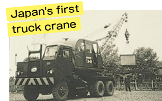
Kobe Steel (currently Kobelco Construction Machinery) 10KT truck crane (1953) Both 10KT (6t) and 20KT (10t) were completed and delivered to the National Police Reserve.
