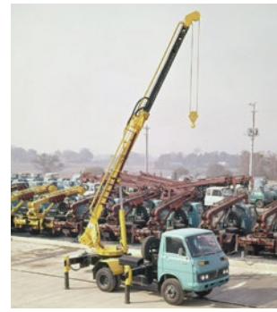
Aichi Sharyo (currently Aichi Corporation) AC-D4Edigger derrick / pole setter (1966) This vehicle consisting of a derrick fitted to a pole setter was a modified version of AC-D4 pole setter.
