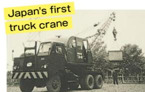
Kobe Steel (currently Kobelco Construction Machinery) 10KT truck crane (1953)
