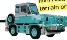
Kobe Steel (currently Kobelco Construction Machinery) RK70M/RK70 mini rough terrain crane (1989)
